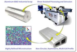
A porthole die configuration is integrated within the rotating ShAPE process to extrude circular, square, trapezoidal, and 2-cell trapezoidal profiles from aluminum alloy 6063 (AA6063) industrial scrap.
