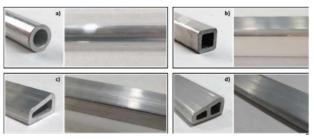
Extrusions made from AA6063 industrial scrap by ShAPE producing (a) circular, (b) square, (c) trapezoidal, and (d) two-cell trapezoidal profiles.
