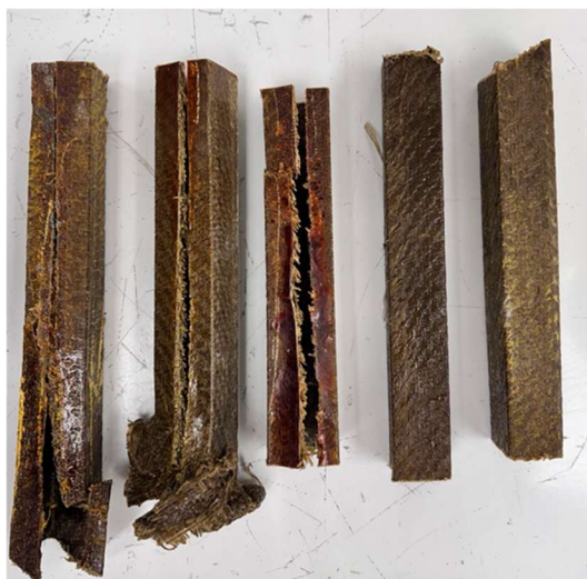
Figure 3. Pultruded square tube using Vitrimax and flax/glass fiber.
